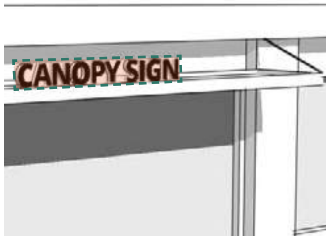
Figure 200-10(2). Area Calculation for Canopy-Mounted Sign
